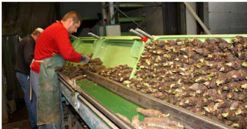
The current process at Endipro is manual. Basically, the process is not ergonomic and also it is tedious and labor intensive due to the repetitive tasks that operators need to perform. Therefore, the Endipro considers automating this process to not only reduce the risk for the operators and improve their working conditions but also reducing the manual labor to increase the overall production efficiency.
