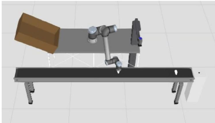
The proposed design can be divided in 3 subsystems; Feeder System, Vision System and Robot System. Figure below illustrates the concept of how these systems would work in coherence and how automated work cell would work.
