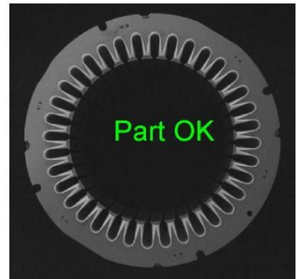
Also, a test setup was made to prove that 2D-vision can help with the correct placement of a motor stator on the mandrel of the slot insulation insertion machine using a cobot.
