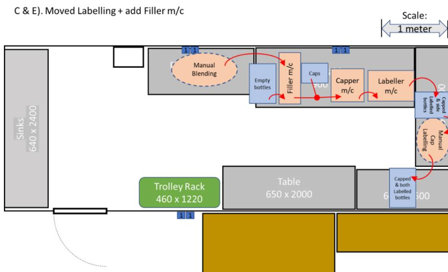
Figure 6. Layout with depositor for filling
