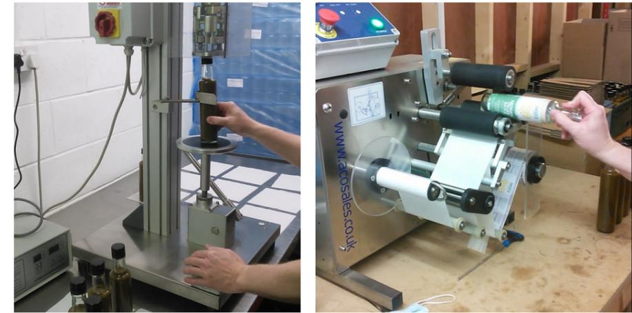
Figure 2. Current semi-automated benchtop capping and side labelling
