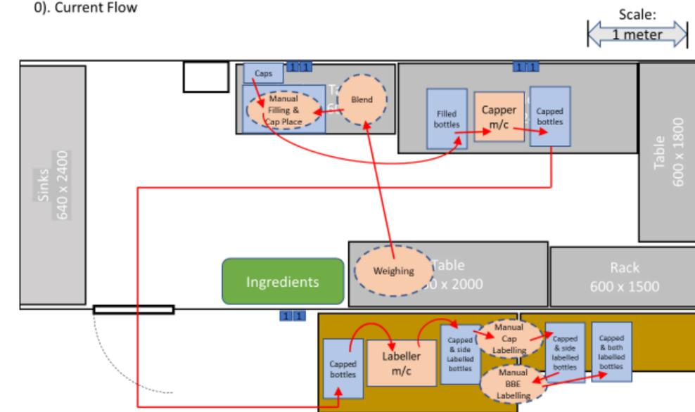
Figure 3. Current Process flow
