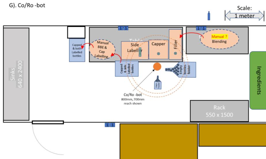
Figure 7. Co/Robotic cell for bottle handling
