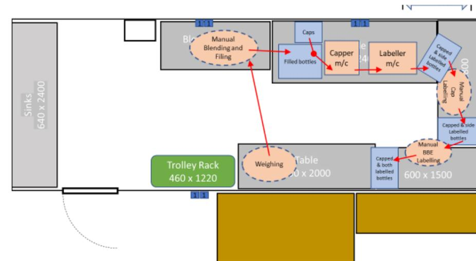
Figure 5. Labelling moved into production space.
